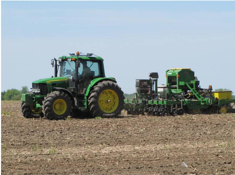
**Figure 2.** Planting of the SMART Project was completed using a Kearney custom 15" planter, capable of applying both liquid and dry fertilizers, as well as a precision control on depth and seeding rate.
