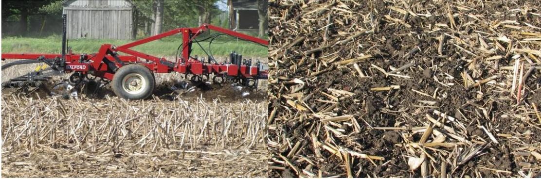
**Figure 1. A Salford RTS tillage unit (right) being operated in a field near Stratford, Ontario. The effects (right) of the Salford RTS on corn stalks and soil after being operated twice. Table 1. The Effects of Tillage on Yield (2011)**
