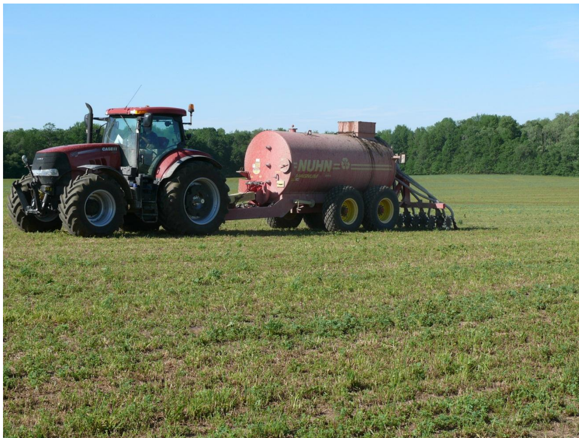
Figure 1: Picture of Manure Tanker with Shallow Incorporation Unit
