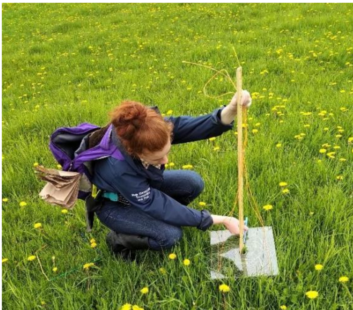
Figure 1. Using a falling plate meter to measure grass bulk height
