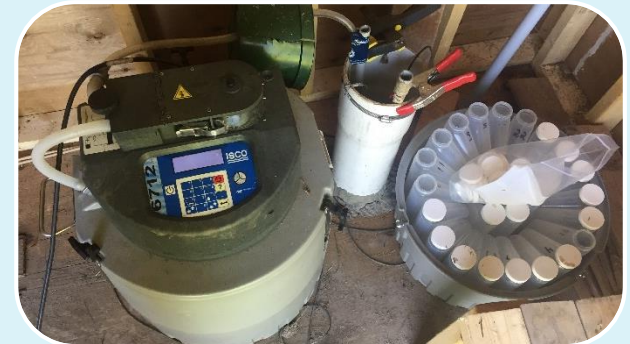
ISCO samplers are used to gather samples from field run-off. Photo courtesy of Maitland Valley Conservation Authority.
