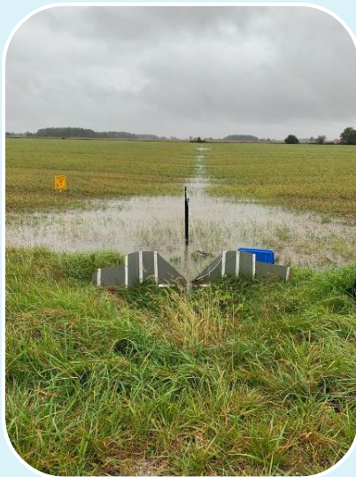
V-notch weirs allow for easier data collection at Henry's site.
