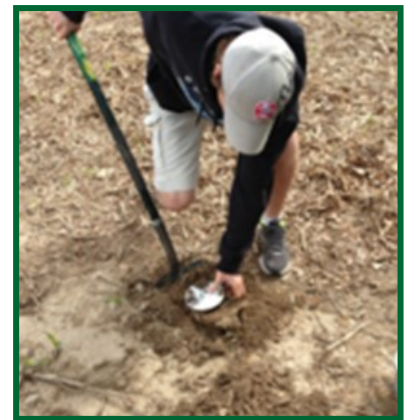
Collecting soil core samples
